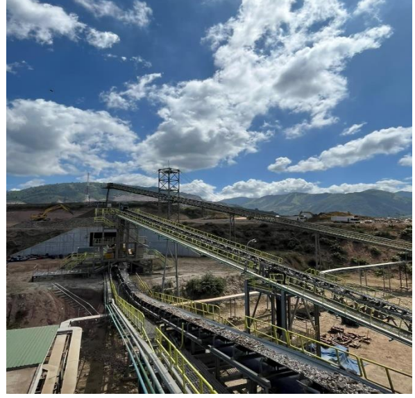
Exhibit 6b. Belt from Jaw Crusher to the next process
