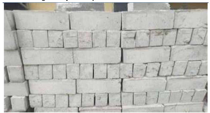
Exhibit 6. Slag which is already converted into bricks
